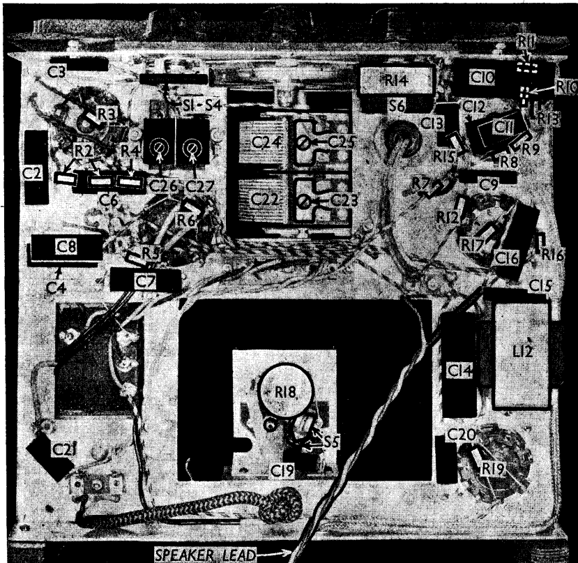
Front view of the unit when removed from the cabinet. A diagram of the SI-S4 unit is on the preceding page. R2 consists of two resistors in series. S5, R18, C19 and the pick-up sockets are on a separate small panel.
