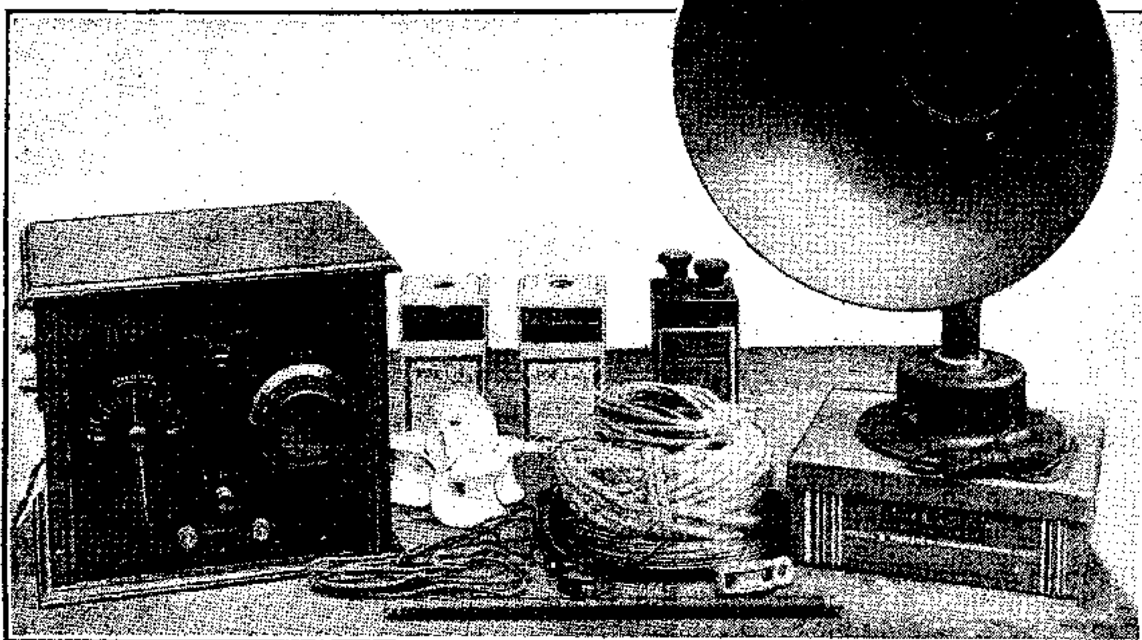
The equipment of the Graves set is unusually complete and includes valves, batteries, loud-speaker and materials for the aerial-earth system.
