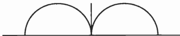
***Fig. 4.9 Radiation Pattern Of A Quarter Wave Vertical.***
