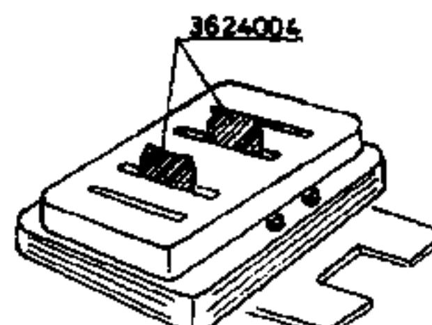
In case the motor has been disassembled it will be necessary to center the rotor. Centering is performed by means of two gauges, supplied together under No 3624004.
