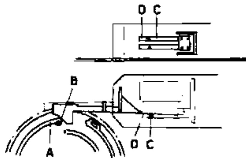
Adjust contact pair C to provide contact when arm B is halfway up on curve segment A when the cam-lifting wheel is rotated manually. Adjustment is performed by bending the tag D through the hole in the relay housing.
