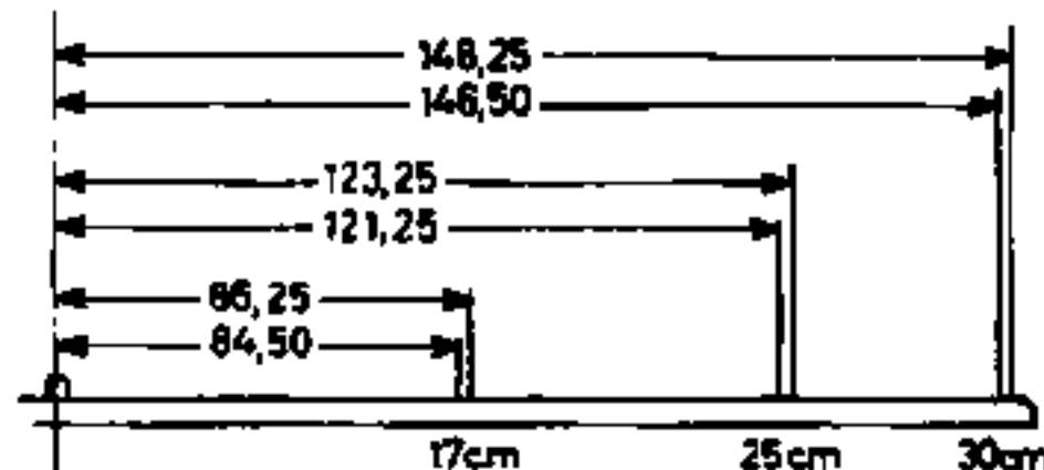
With the record selector at "17", adjust eccentric A so that the pickup when operated by the automatic cueing mechanism will lower into the field marked "17" on the sketch above.
