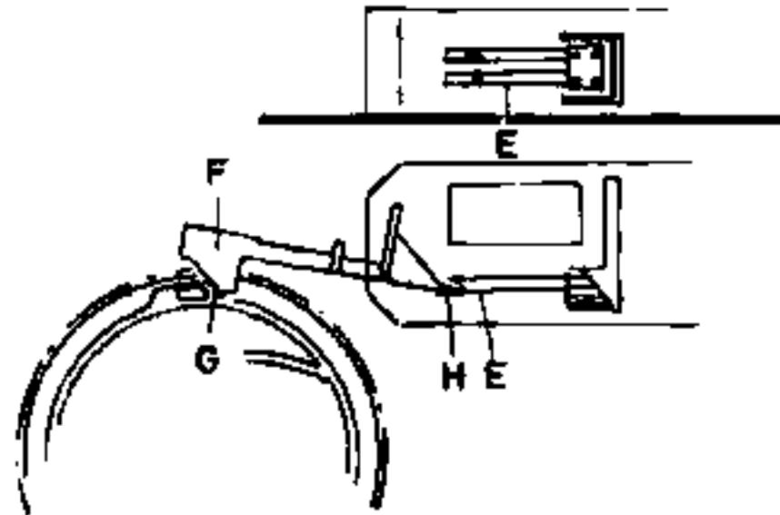
Adjust contact pair E so that relay holding voltage is switched off when arm F is halfway up on cam G.
