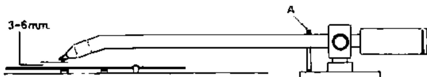
Lifting screw A is adjusted with the pickup arm raised and the pickup stylus floating between 3 and 6 mm above the turntable's outermost knobs (see sketch).
