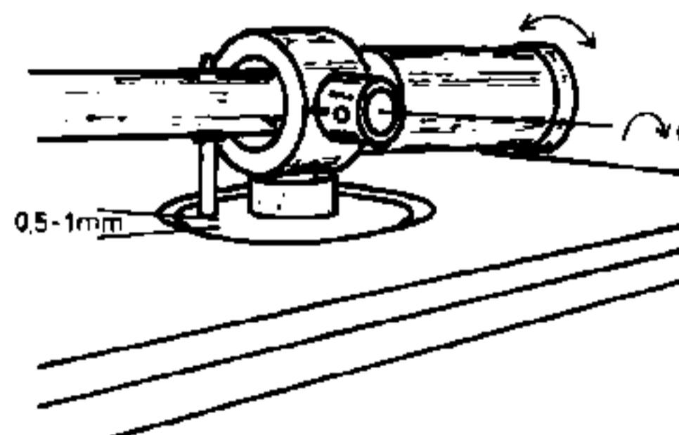
Turn the stylus-force adjustment screw to 0.
