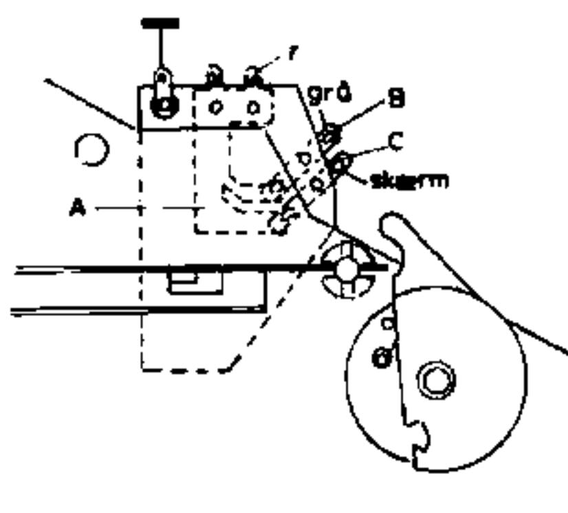
Adjust tags B and C so that on the pickup being raised contact will first be made between A and B (short-circuiting the channels together) and thereafter between A and C (Short-circuiting the signal).
