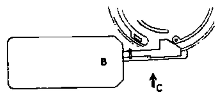
Adjust relay B as far as possible in the direction of arrow C but only to the point where the relay will positively attract the armature when the LIFT button is pressed quickly.
