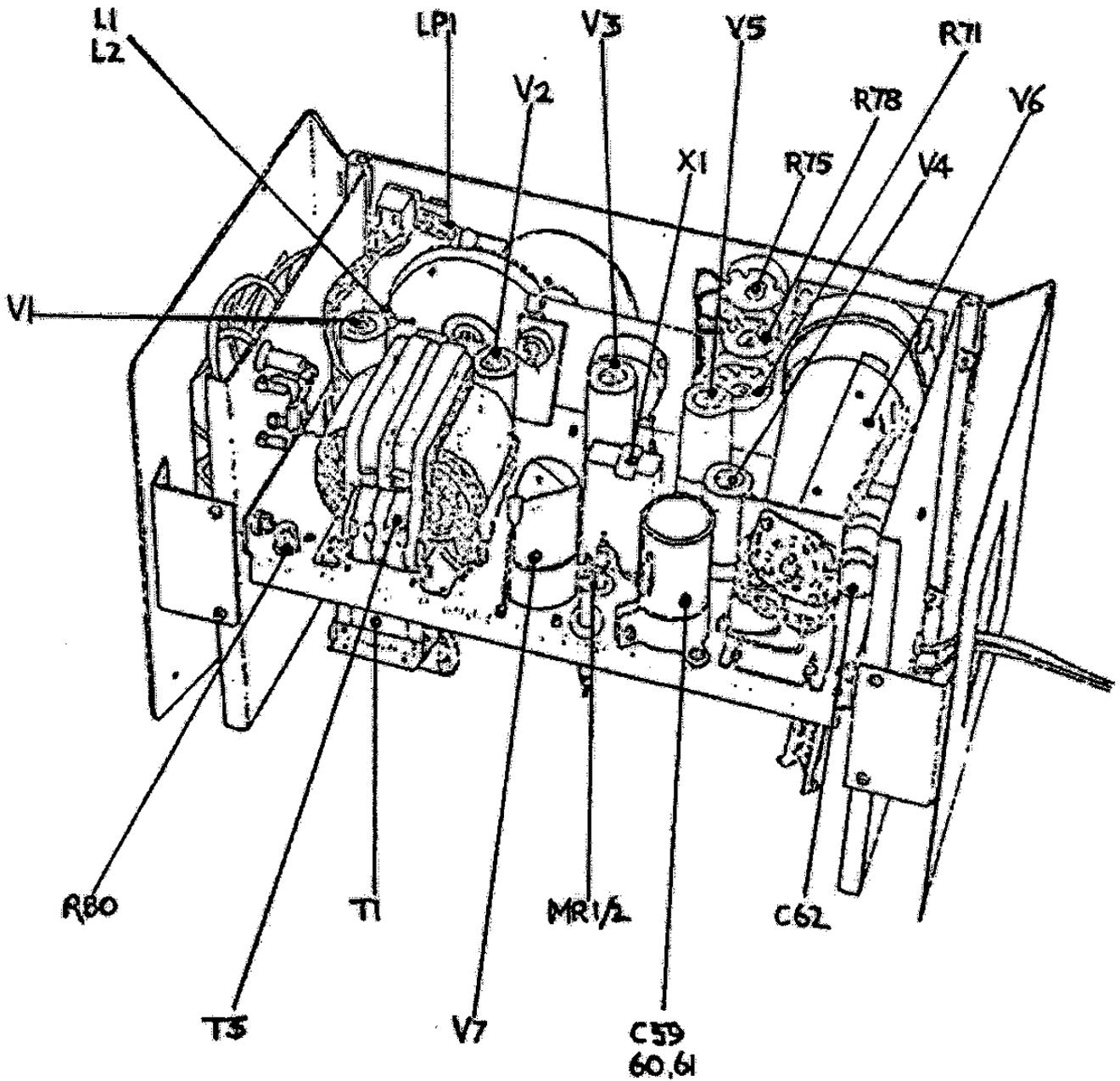
FIGURE 2b RADIVET TYPE 211 TOP VIEW
