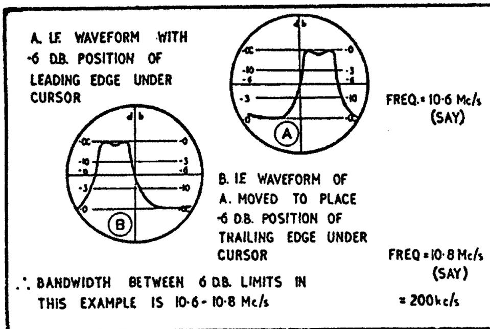
Figure 3. Bandwidth measurement of I.F. response curve.
