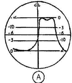
IF WAVEFORM OF (A) MOVED TO PLACE -6db POSITION OF TRAILING EDGE UNDER CURSOR
